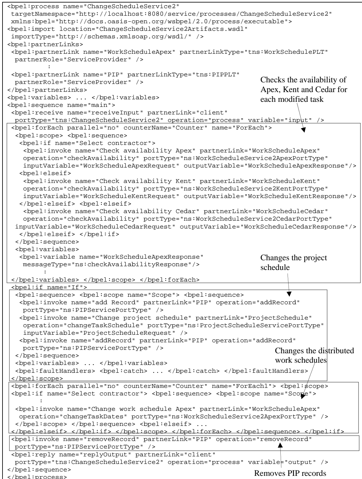
Figure 4.25: BPEL process that changes the project schedule and the distributed work schedules in the scenario demonstration
