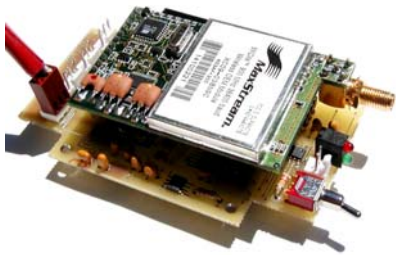
Figure 1. Fully assembled wireless sensing unit prototype (battery and external container not shown for clarity).
