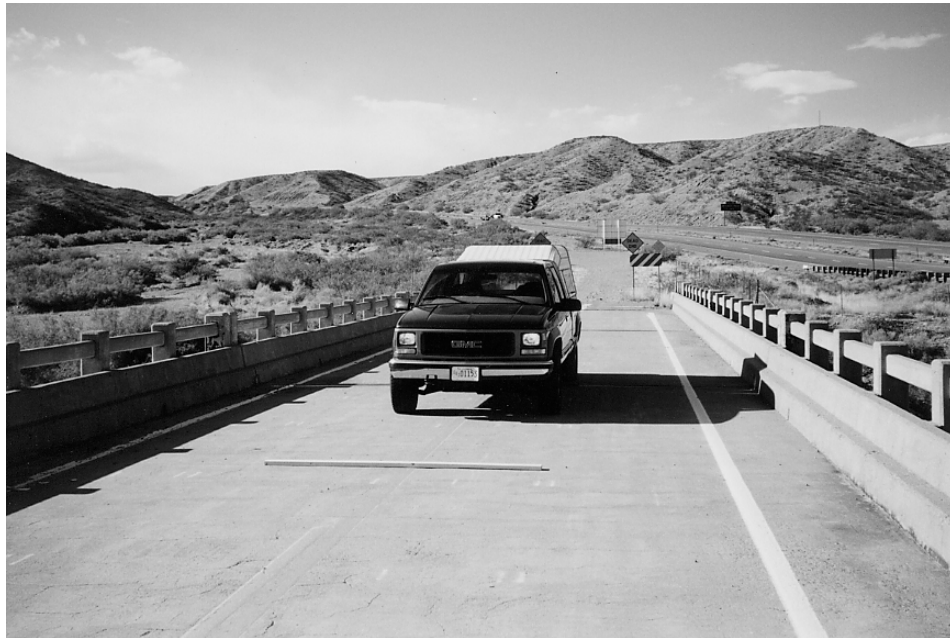
Figure 4-35: Forced vibration test of a speeding truck driving over a wood stud
