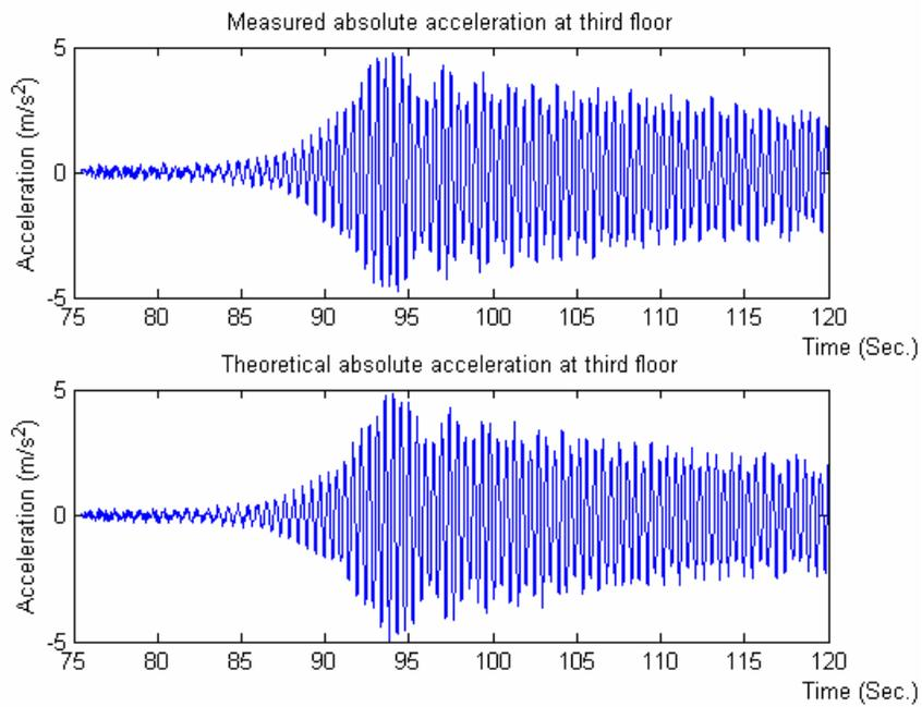
Figure 8 – Comparison of measured and theoretical absolute acceleration at third floor
