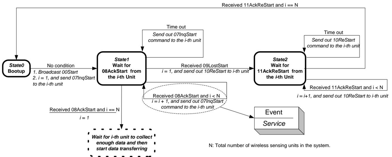
Figure 3 – Abridged communication state diagram for the central server
