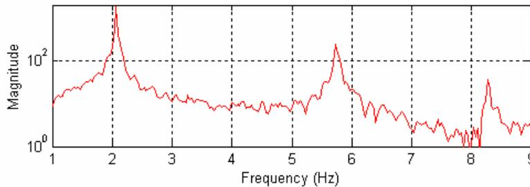
Figure 6 – Discrete Fourier Transform of the third-floor acceleration during free-vibration
