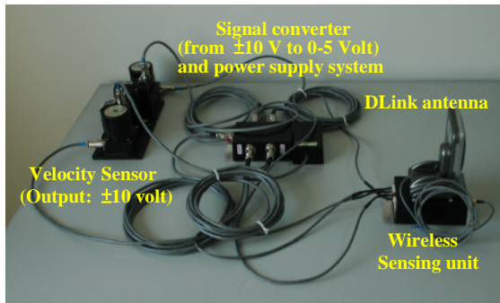
Fig.3: A signal converter between the velocity meter and the wireless sensing unit.
